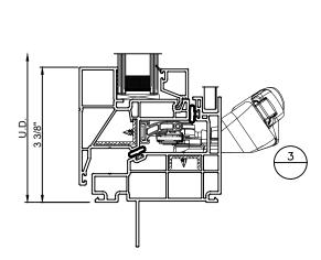
V300 **SERIES** NARROW FIXED OVER AWNING CONFIGURATION INSTALLATION METHOD NAIL FIN HORIZONTAL C-MULL
